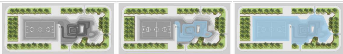
Fig. 28. Top view of the pilot water square - during dry periods, medium rain, and heavy storms (left to right) (© De Urbanisten).
