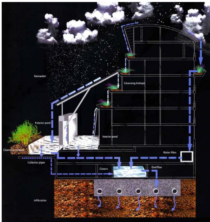
Left: Fig. 78. Rainwater concept for Prisma includes facilities for collecting, storing, purifying and infiltrating (© Atelier Dreiseitl). Right: Fig. 79. In Nuremberg Prisma, rainwater is used for natural air conditioning, fire fighting and irrigation (© Atelier Dreiseitl).
