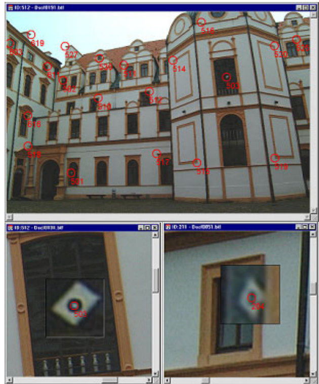
Fig. 4: Image point measurements of tie points (upper) and control points (lower) in one image of Celle castle
